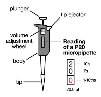
The volumes that a micropipette can accurately dispense are written on it. In this activity you will be using either a P20 or P200 micropipette, which can accurately dispense between 2 and 20  $\mu$ L (P20), or 20 and 200  $\mu$ L (P200), of liquid. Setting the volume outside of this range can damage the accurately calibrated mechanisms inside the micropipette.
